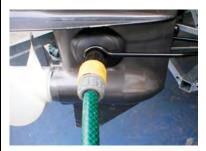
**Step 5:** Hook up the motor flusher to the Out-Drive like the picture to the left. Place the motor flusher over the in-take vent on the out-drive. Look for about three to five round drill holes. This is where the engine sucks the lake water into the boat motor.
